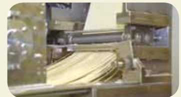
Different cutting teeth are used for different kinds of noodles. In order to avoid contamination, the teeth are tipped with resin.
