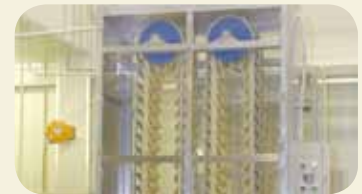
Noodle belt conditioning in the proprietary special conditioning box
