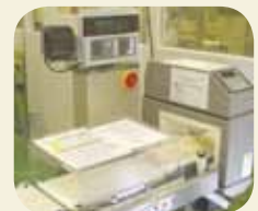
If any products have abnormal values, they are automatically removed from the line.
