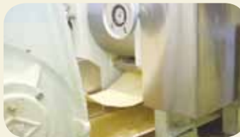
Compounding is repeated depending on the type of noodle. This process determines the firmness of the noodles.
